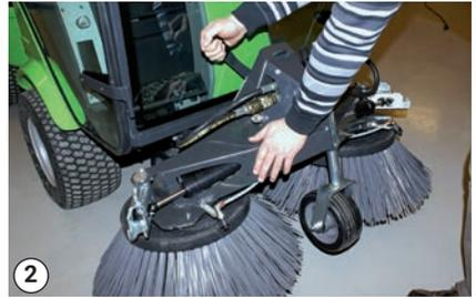
Tilt the attachment into the machine
