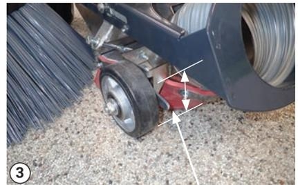
Adjusting the rubber to the ground
