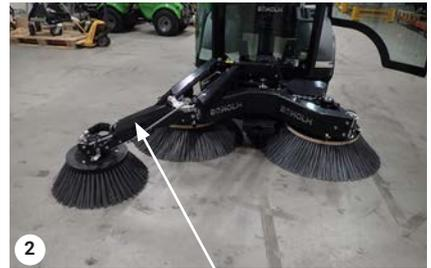
Remove shield (brush in out position)
