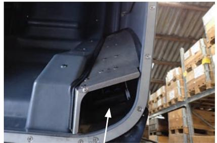
Remove hatch on each filter
