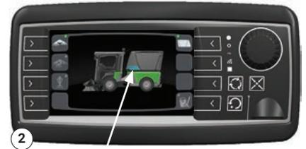
Tank gauge (the selection screen of the hopper)
