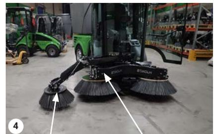
Tilt (left joystick) Move arm (right joystick)
