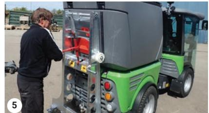
Push the Attachment frame and ensure the hooks are in place in the lifting devices.
