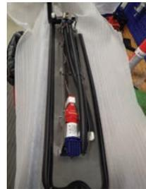
Recycling filter and pump assembly.
