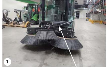
Adjusting lifting point (M10 nut)
