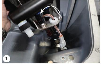
Turn to side and pull out. Connector hole
