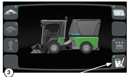
Press and hold the “bucket” for 3 sec. until the green light turns on.
