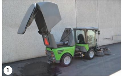
Tip waste tank completely
