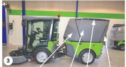
Fresh water tank Waste tank Cap Rear cover
