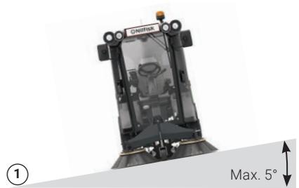
1 Do not drive on slopes with an incline of more than 5°
