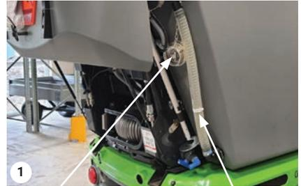
Open filter coupling fill water to min. Water lable (approx. 125 L)
