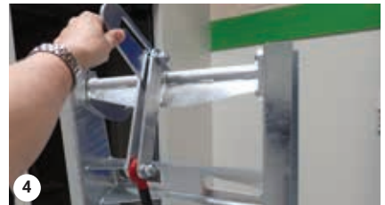
Press up the hook lift arm
