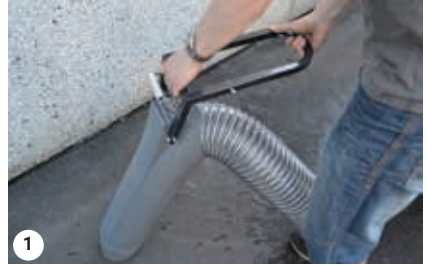
Use external hose to clean system
