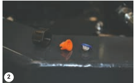
Take out filter and nozzle and clean
