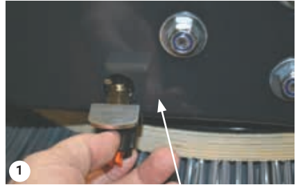
Unscrew nozzle nut
