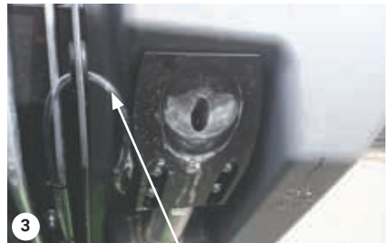
Detach hose, drain leftover water
