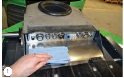
Clean the snap couplings with a cloth
