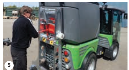
Push the Attachment frame and ensure the hooks are in place in the lifting devises.
