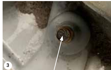
Clean the steel filter at the vacuum
