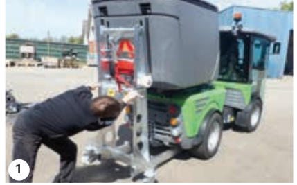
Fitting the hopper
