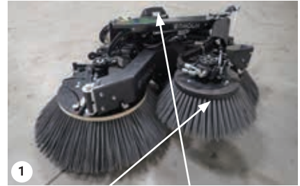
Side brush lifting point
