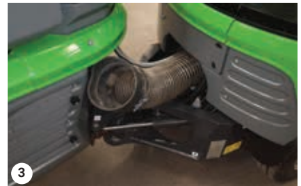
Clean hose at the articulation joint
