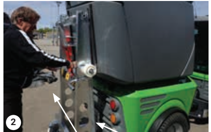
Lower the hopper on to the frame with the ratchet load carrier
