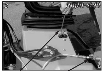
DTap for front-mounted jet sprayers
