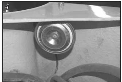
Ensure connector is connected to speaker
