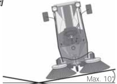
Do not run the machine on slopes or inclines exceeding 10°
