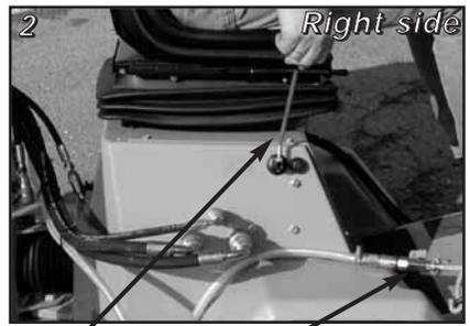
DTap for front-mounted jet sprayers
