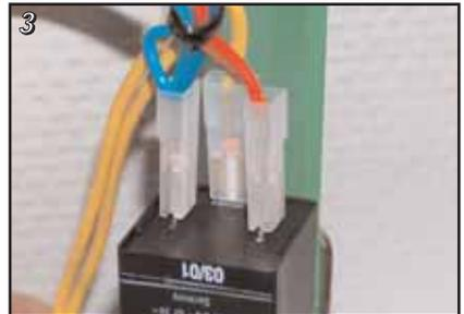
Check the pins on the relay
