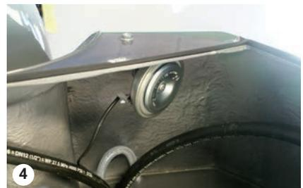
Ensure connector is connected to speaker
