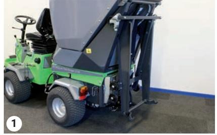
Transporting the hopper frame on the hopper
