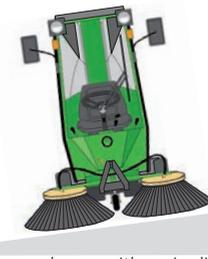
Do not drive on slopes with an incline of more than 10°
