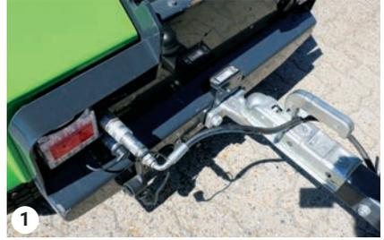
Connect trailer coupling, hydraulic hose (and electrical plug, if available).
