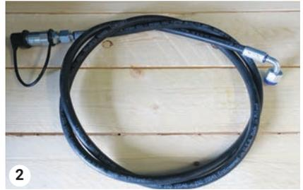
Coupling mounted in the straight end, on the shortest hose.
