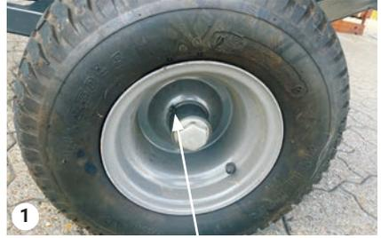
Grease greasing points in the wheels.
