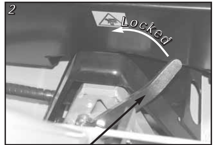
Locking handle on the A-frame - open
