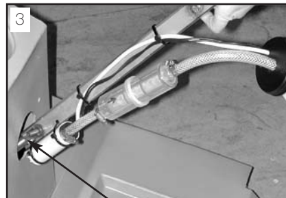
Be careful not to damage the level sensor
