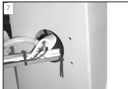
Tie together the pump and the fittings with a hose clip in the same height
