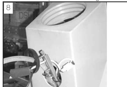
Remount the pump arrangement
