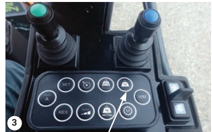
Activating weight distribution (c)
