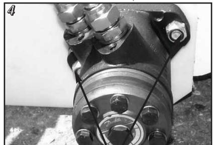
Loosen the bolts that hold the oil motor in place
