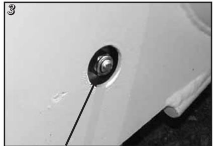
Loosen the bolt that holds the roller brush in place
