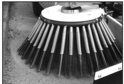
The machine must be in motion while the brush is rotating.
