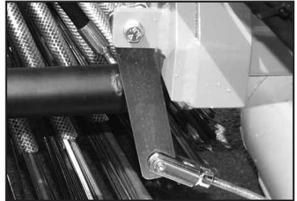
2-3 mm gap between the metal and the A-frame
