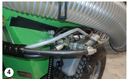
Mount hydraulic hoses to D connectors
