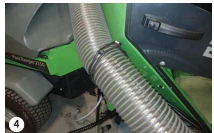
Hose fixed to cabin with rubber mount
