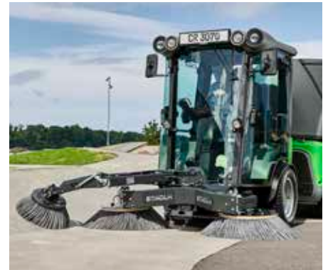
Suction sweeper with 3rd side brush
