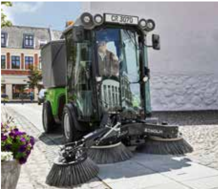
Suction sweeper with 3rd side brush
